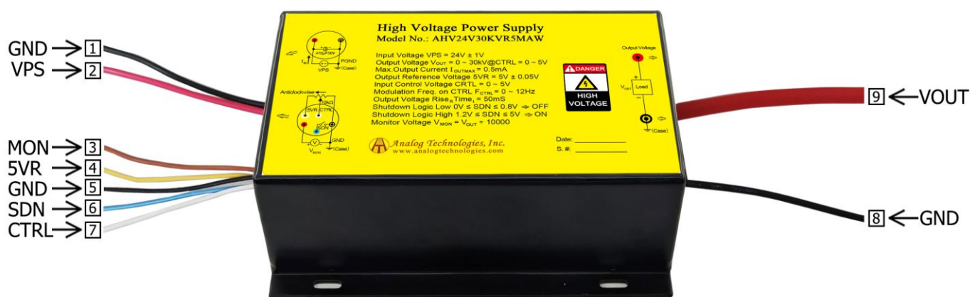
Figure 2. The Connecting Lead Wires of AHV24V30KVR5MAW
