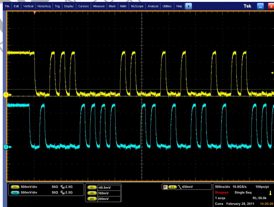
Figure 5. EMI4192 MIPI D-PHY LP Mode Measured Results
