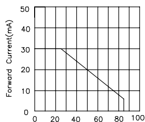
Ambient Temperature TA(°C) FORWARD CURRENT DERATING CURVE
