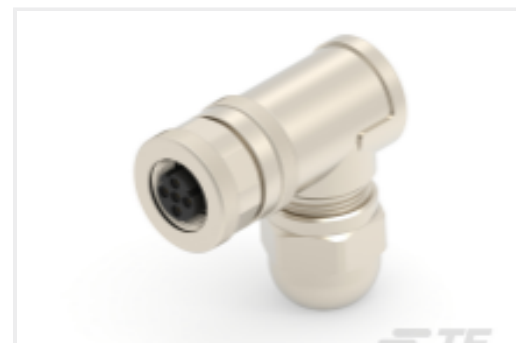
TE Part #T4112511051-000 M12 F, 5P GOLD D_CODE RA SHIELDED PG7
