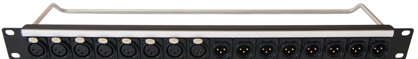
CP30183 - 1U Panel loaded with 8 x XLR 3DCF + 8 x XLR 3DCM. M3 Holes. Front mounted. Solder tag.
