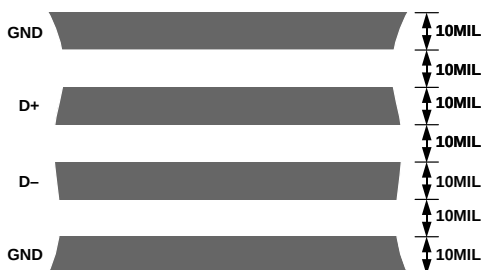
Figure 18. Arrangement of Signal Tracks
