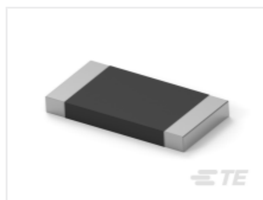
TE Part #4-2176421-4 TLRP 2512 2.0W R005 1% 50PPM 4K RL
