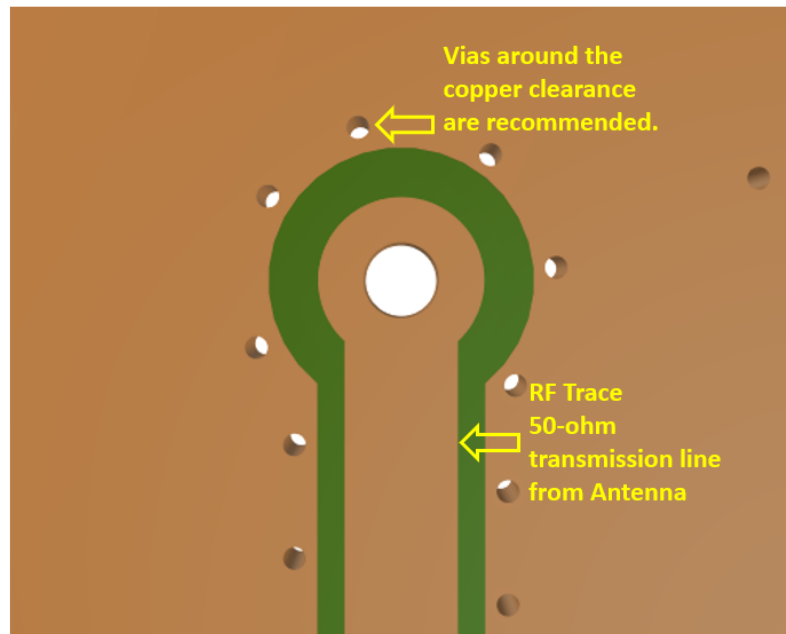
Bottom view of the PCB Reference Design, showing transmission lines and integration notes.
