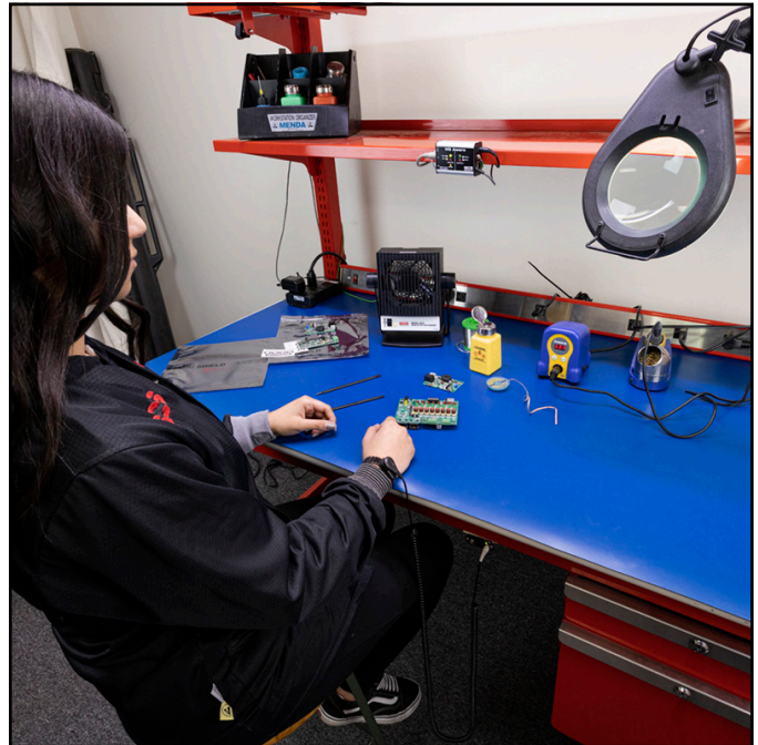
Figure 11. Using the SCS 770069 Power Relay to supply power to a workbench when the operator is properly grounded
