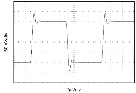
SMALL-SIGNAL STEP RESPONSE
